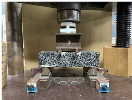
Fig.5 View of the flexural strength test
