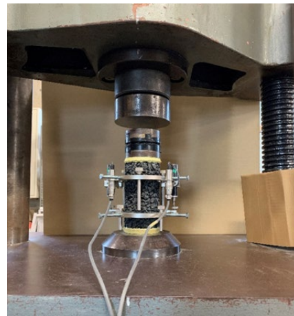
Fig.4 View of compressive strength test
