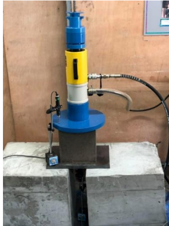
Fig. 1: Experimental set-up for pull-out test
