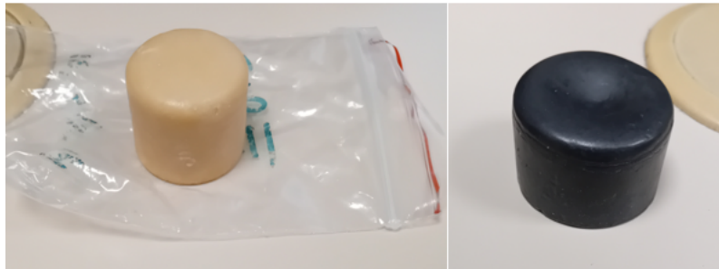
Fig. 3. samples, (a) pure beeswax (b) beeswax 10 w% graphite composite
