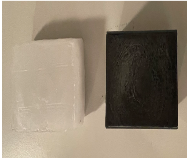
Fig. 2. samples, (a) pure paraffin RT55, (b) paraffin 10 w% graphite composite
