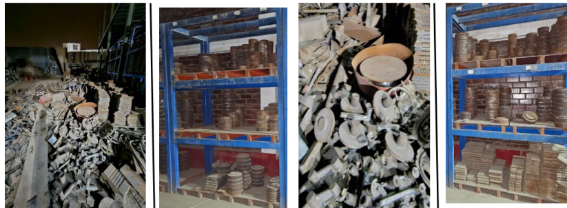
Fig. 5: Before and after implementation Seiri and Seiton
