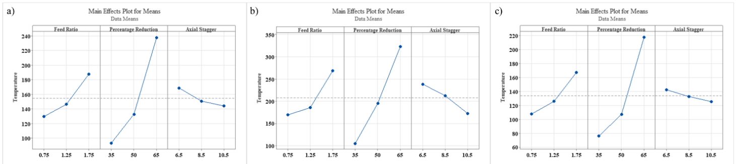
Fig. 9: Main Effective Plots for Temperature on a) MDN-250, b) 15CDV6, c) AISI 4130
