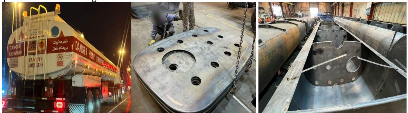
Figure 6: the oil tanker benchmark with built in baffles, Mula company Kuwait.
