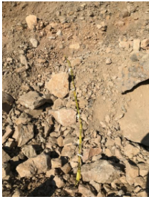
Fig. 5 Real post blasting stockpile
