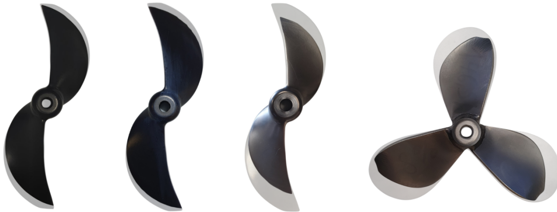
Fig. 5 Pictures of propellers before (gray) and after wear tests. From left to right: Phantom Physinit® 80 g/l; Phantom Physinit 200 g/l; Phantom stainless-steel 80 g/l; three-blade stainless-steel 80 g/l
