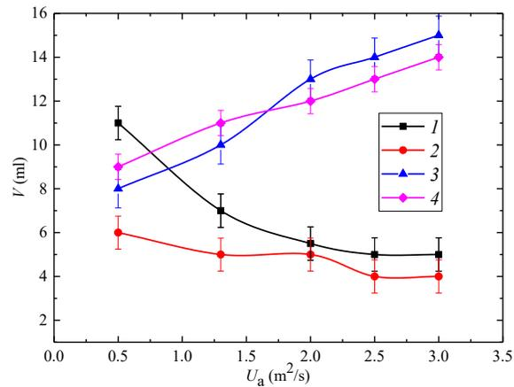
Fig. 3: Dependence of the minimum volume of extinguishing liquid necessary to suppress the flame combustion and thermal decomposition of FFM on air flow velocity at burning different types of FFM: 1 – needles, 2 – leaves, 3 – a mixture of FFM, 4 – herbaceous plants.
