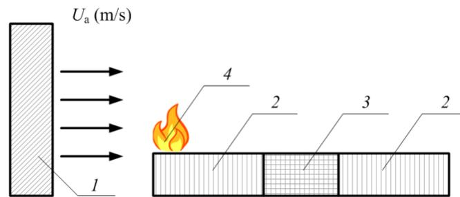
Fig. 1: Experimental scheme: 1 – air blower, 2 – dry FFM, 3 – barrier line; 4 – initiation of combustion.
