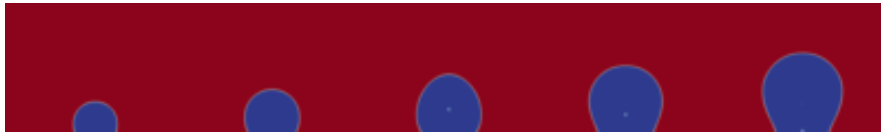
Fig. 2: Evolution of the bubble formation. Results for a constant heat flux ( 1900 \text{ W/m}^2 ) and a contact angle of 159^\circ .
