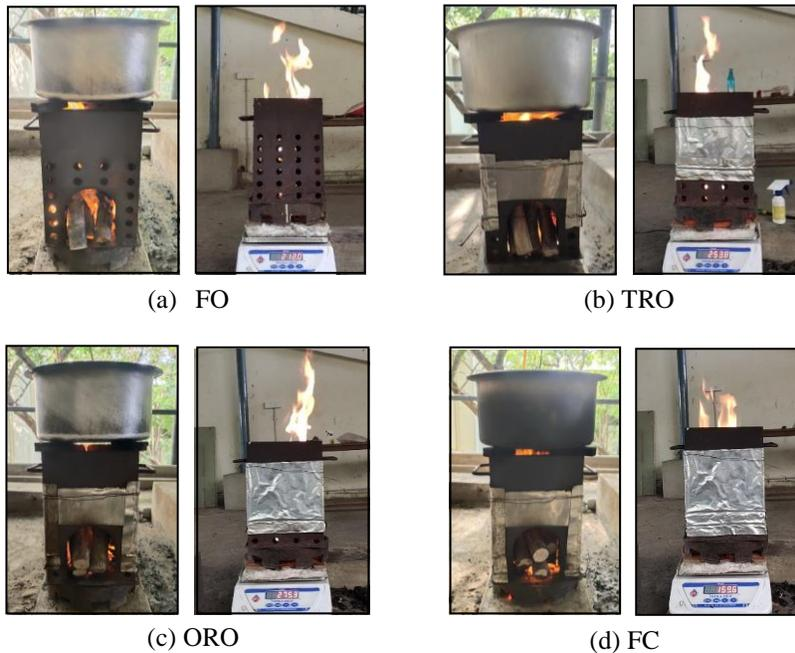
Fig. 2: Experimental setup for different ventilation conditions of wood stove (a) FO (b) ORO (c) TRO and (d) FC
