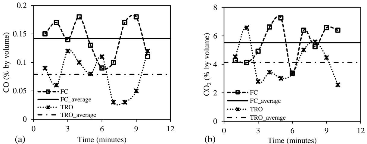
Fig. 4: Variation of CO<sub>2</sub> and CO during steady burning for fully closed (FC) and two rows open (TRO) cases
