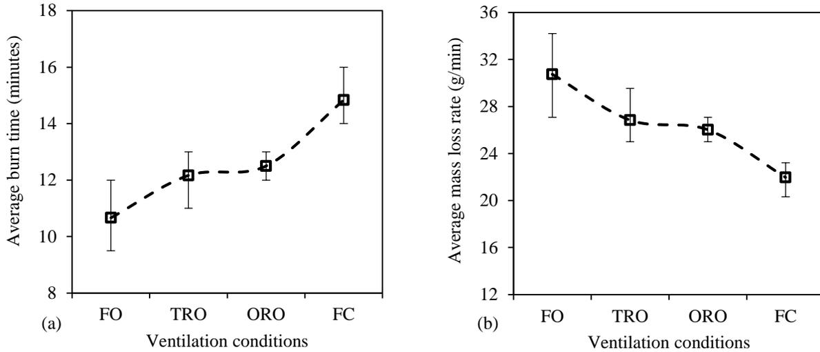
Fig. 5: (a) Average burn duration and (b) average mass loss rate for wood stove with different ventilation conditions
