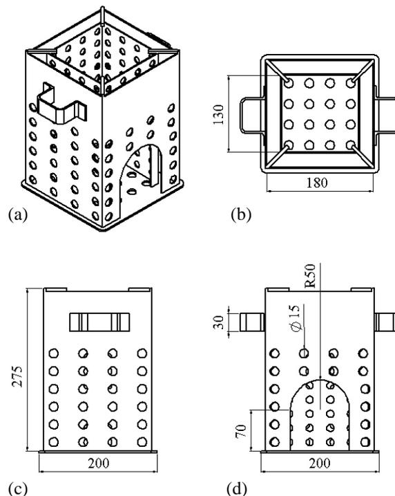
Fig. 1: Geometry of wood stove (a) Isometric view (b) Top view (c) Side view and (d) Front view. All dimensions are in mm
