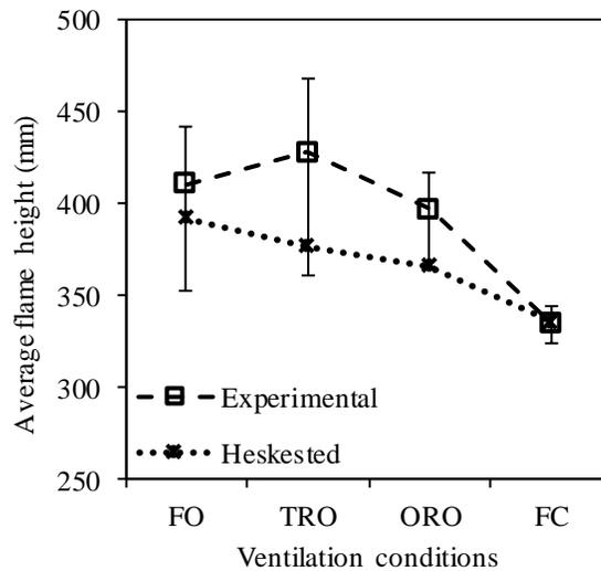
Fig. 6: Average flame height with different ventilation conditions
