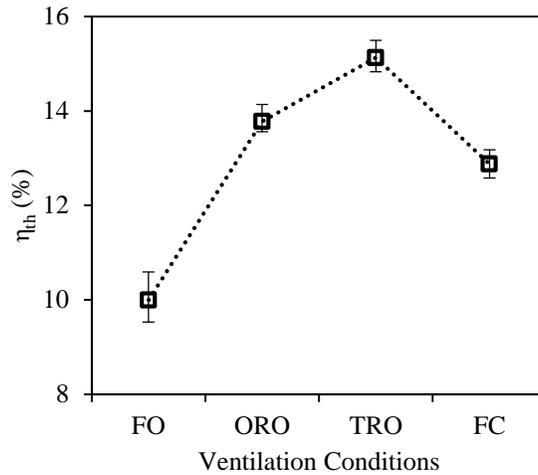
Fig. 3: Average thermal efficiencies for different ventilation conditions
