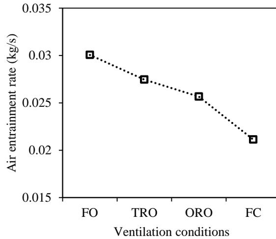
Fig. 7: Air entrainment rates for different ventilation conditions
