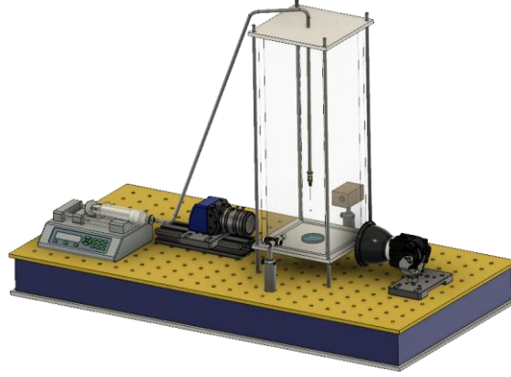
Fig. 1: Schematic of the experimental setup characterizing the droplet dynamics.
