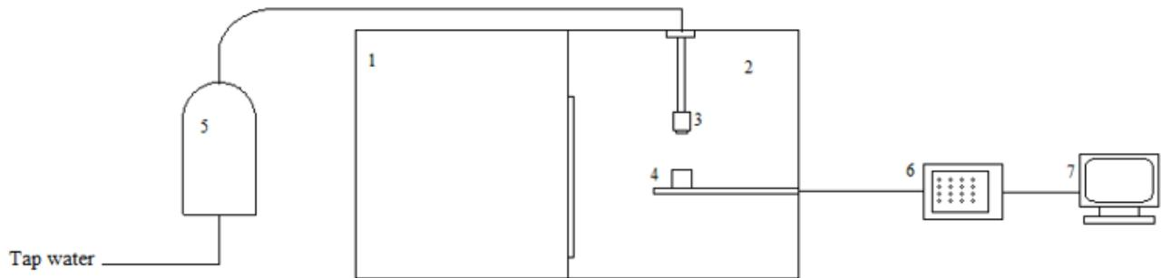
Figure 1: Measuring stand: 1- electric resistance furnace, 2 – cooling chamber, 3 – nozzle, 4 – cylindrical sensor, 5 – water tank, 6 – data acquisition system, 7 – computer.
