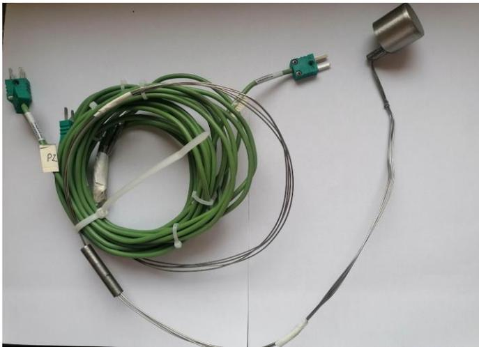
Figure 2: Sensor, made of Inconel with thermocouples.
