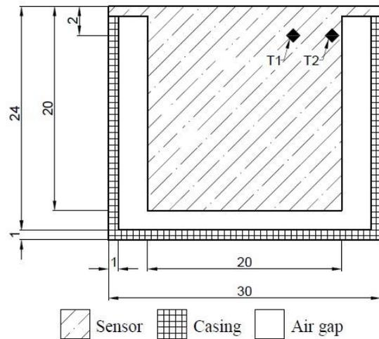
Figure 3: Diagram of the sensor with the location of the thermocouples (T1, T2).
