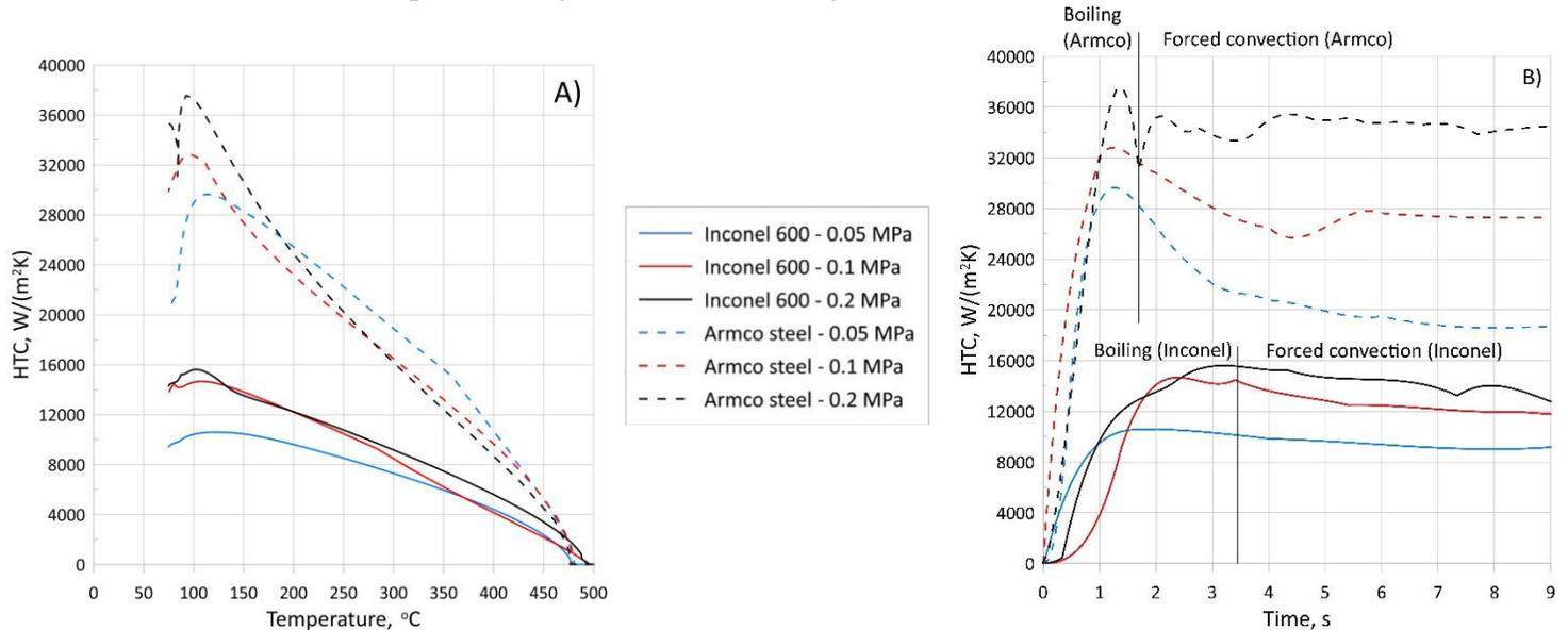
Figure 4: Average HTC value on the cooled surface as a function of surface temperature (A) and time (B).
