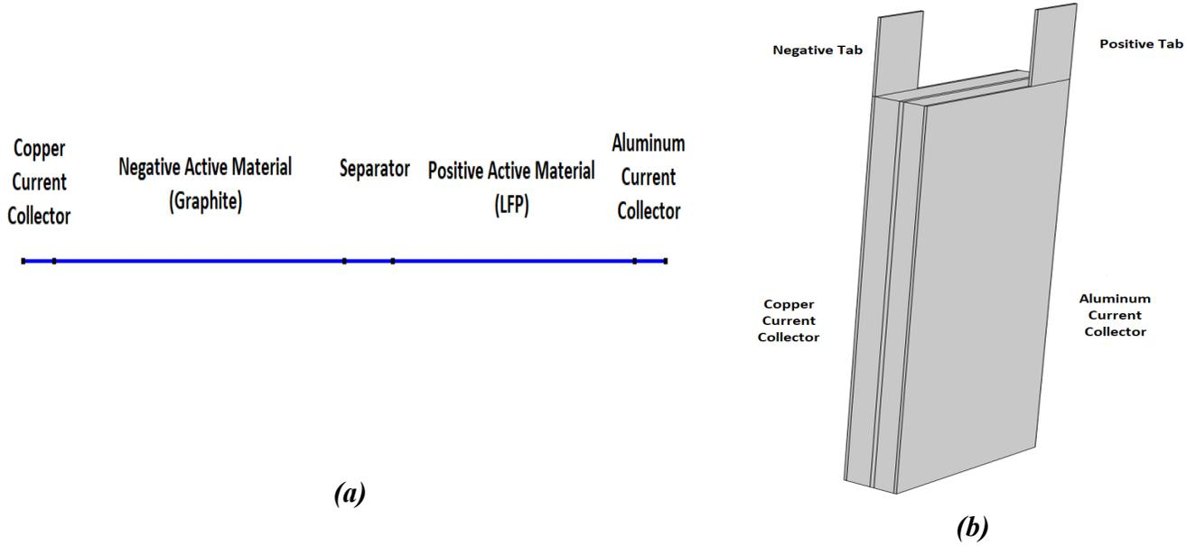
Fig. 3: Schematic of 1D (a) and 3D (b) li-ion cell geometry.
