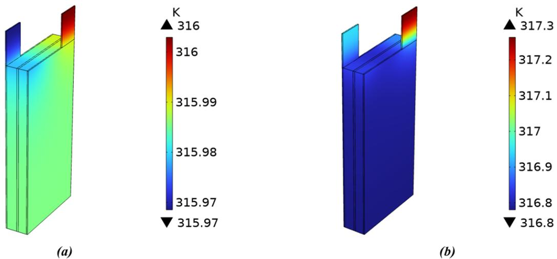
Fig. 6: 1 layered cell temperature distribution at the end of 1C charge, (a) 1D EC, (b) 3D EC.
