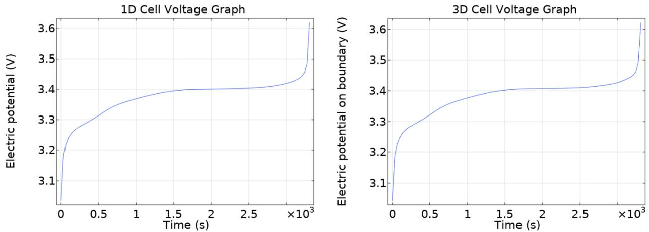
Fig. 5: 1D and 3D one layered cell voltage change at 1C charge.
