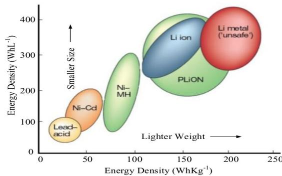
Fig. 1: Volumetric (Wh/L) and gravimetric (Wh/kg) energy density of various battery types [1].
