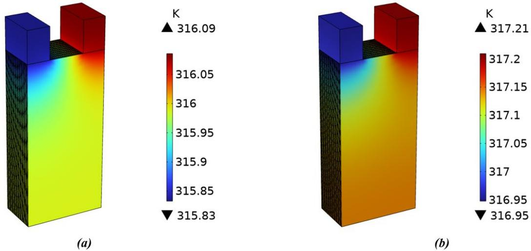
Fig. 7: 20 layered cell temperature distribution at the end of 1C charge, (a) 1D EC, (b) 3D EC.
