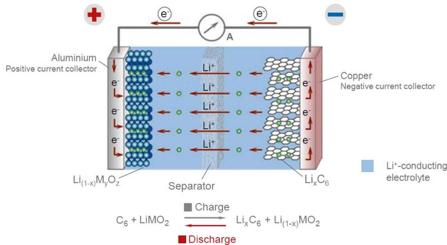
Fig. 2: Schematic representation of the movement of ions and electrons during discharge of a li-ion battery [3].
