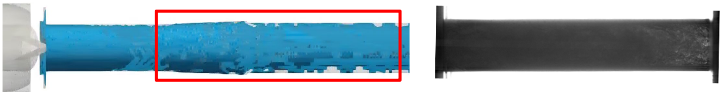
Figure 7: Test p6 at 55° aperture: (right) void fraction field from CFD simulation (left) video frame from high-speed imaging.
