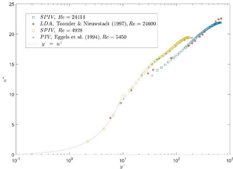
Fig. 3: Mean streamwise velocity profiles in inner units at Reynolds numbers of 4928 and 24414 obtained with SPIV, compared with the results of DenToonder & Nieuwstadt [4] and Eggels et al [5].
