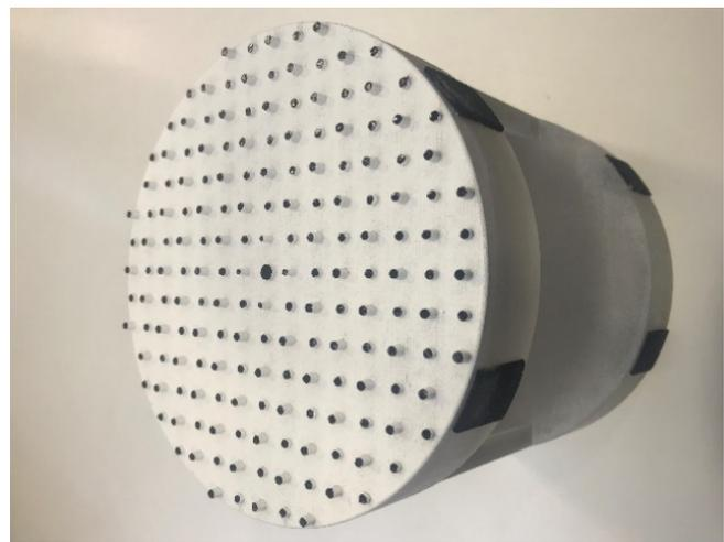
Fig 2.: Two-level calibration target used for the spatial calibration of the SPIV system, as seen by the right camera.
