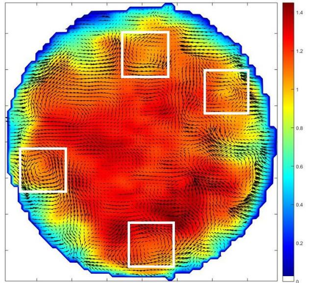
Fig. 4: Instantaneous vector field of  $Re = 24414$  with highlighted streamwise vortices. Colors indicate the magnitude of the streamwise velocity component normalized by the bulk velocity.
