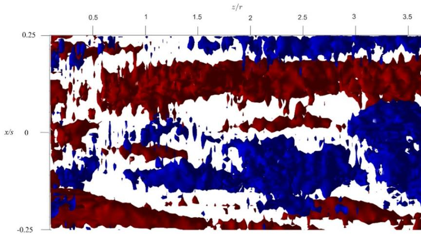
Fig. 5: Velocity fluctuations along the mean flow direction (flow from left to right) obtained at  $Re = 4928$ , where the red isocontours show velocities above 1.1 times the local  $U_{\text{mean}}$  (the turbulent  $U$  profile of all acquisitions), while the blue isocontours represent velocities below 0.9 times the local  $U_{\text{mean}}$ .
