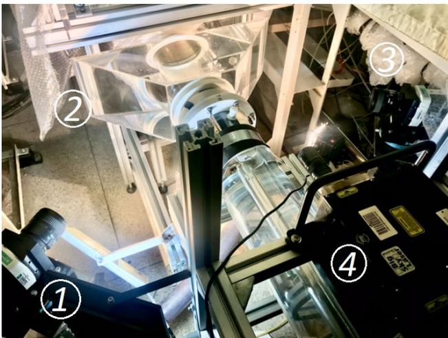
Fig. 1: Visualization section, numbers indicate the positions of cameras (1 & 3), Laser (4) and trapezoidal water-box (2).
