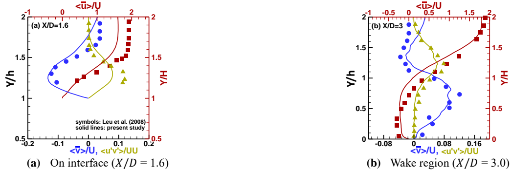
Fig. 3: Comparison of first- and second-order velocity statistics obtained from the pore-scale Large Eddy Simulation study with experimental measurements by Leu et al. [21]. The symbol \langle \bar{\cdot} \rangle denotes the time-averaged value of the filtered variable.
