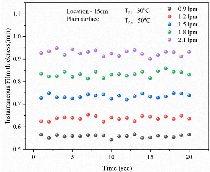
Fig. 3: Variation of Instantaneous Film thickness with time
