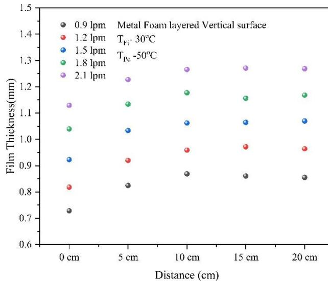
Fig. 5: Film thickness variation along the length of the Metal Foam layered plate
