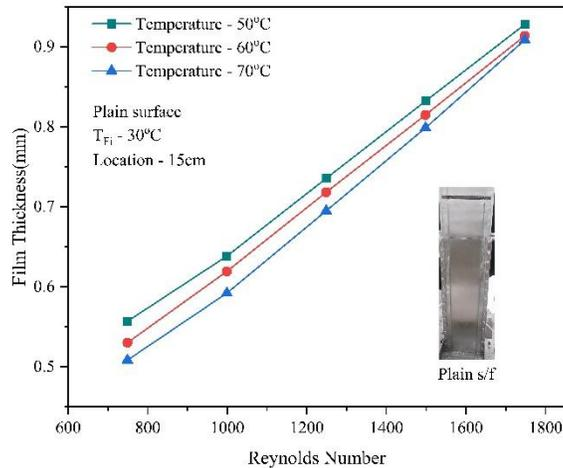
Fig. 8: Film thickness variation due to different plate surface temperature
