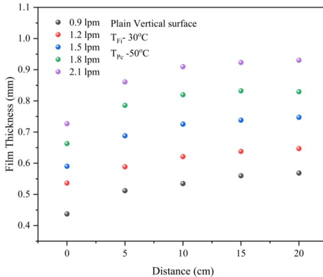
Fig. 4: Film thickness variation along the length of the Plain plate
