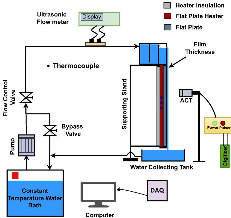
Fig. 1: Schematic diagram for film flow on vertical surface.
