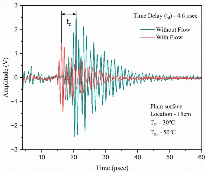
Fig. 2: Shift in signal with and without flow
