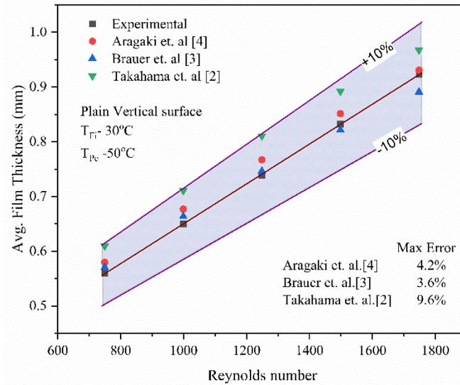
Fig. 6: Validation of Experimental data with correlation
