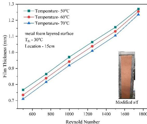
Fig. 9: Film thickness variation due to different plate surface temperatures with Copper foam
