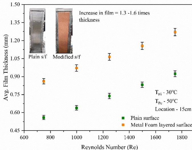
Fig. 7: Film thickness variation for plain and modified surface with Reynolds number
