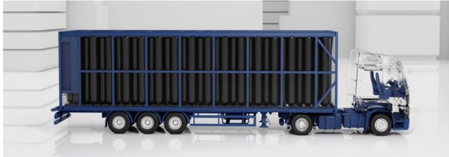
Fig. 1: Illustration of a containerised Bulk Gas Transport system with vertically-oriented cylinders in a staggered array.
