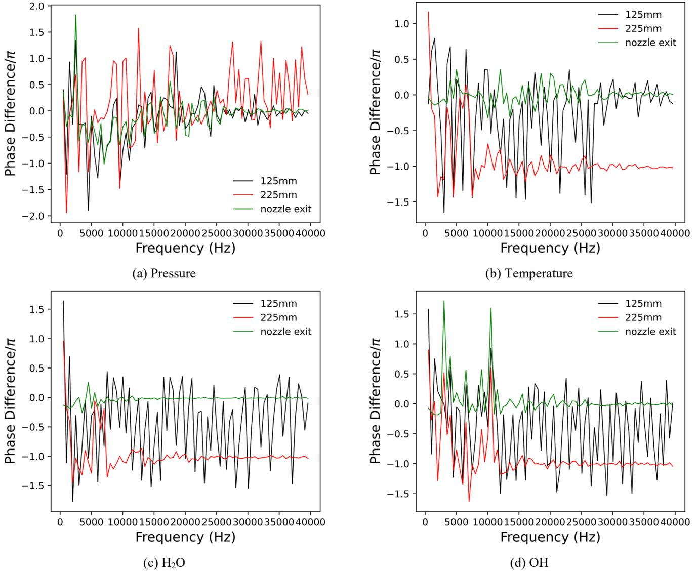
Fig. 3: Compared to the phase difference at nozzle inlet
