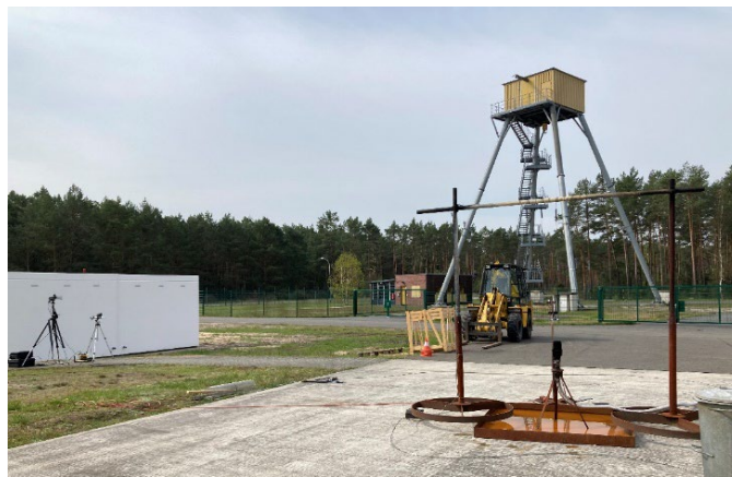
Fig. 3: Baseline open nozzle experiment setup. Video camera and infrared camera were located to the south of the open nozzle.
