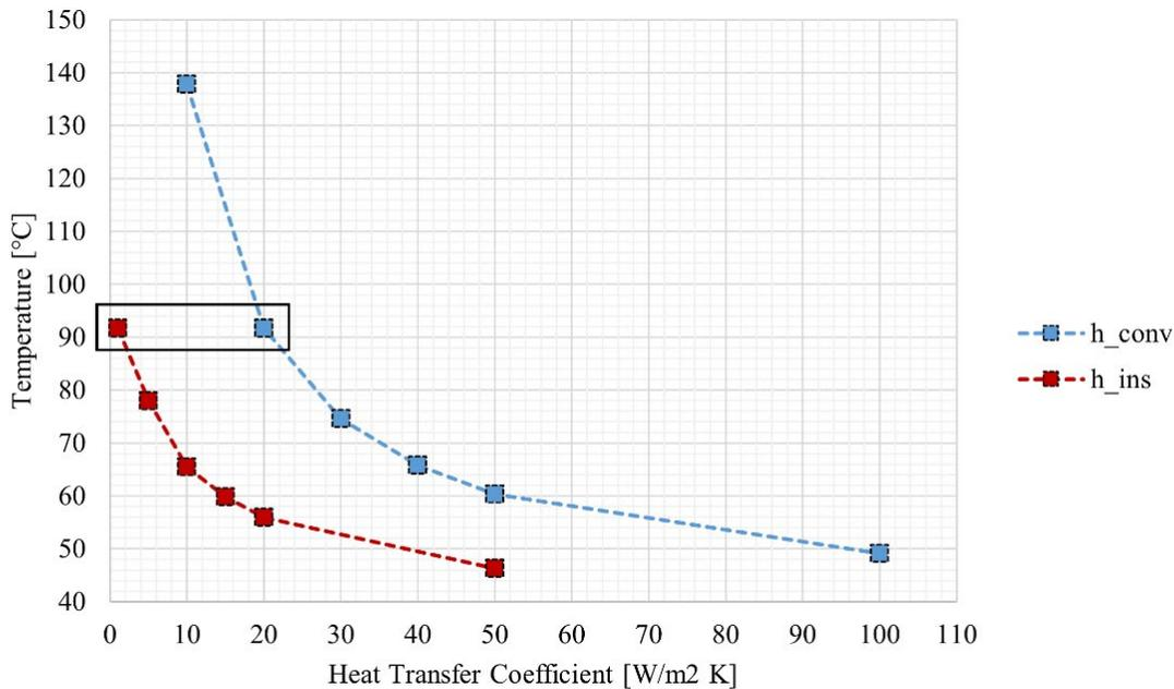
Figure 6: Effect of equivalent heat transfer coefficients on volume average battery temperature for convection wall (heat sink) and insulation wall, as defined in Figure 2. The dark square points to the benchmark values assumed in previous simulations, i.e. 20 W/m<sup>2</sup> K and 1 W/m<sup>2</sup> K for convection and insulation walls, respectively.
