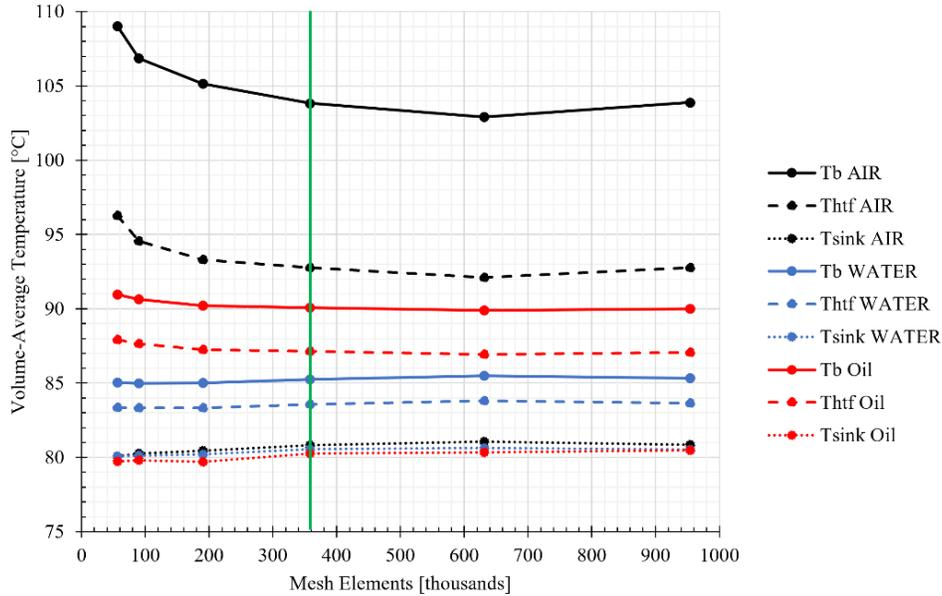
Figure 4: Mesh sensitivity analysis on volume-average temperatures of battery, HTF, and heat sink for three different HTF.
