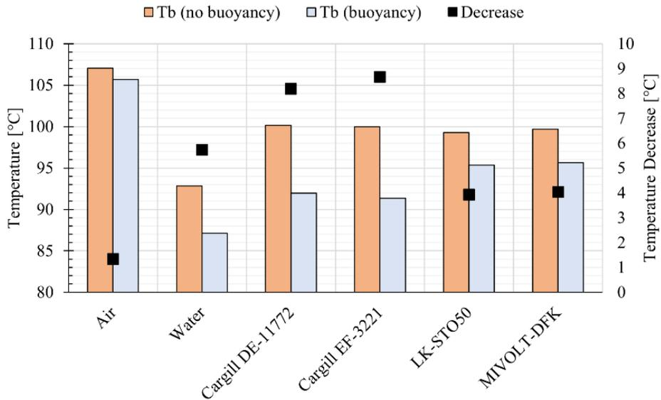
Figure 5: Steady-state average volume temperatures of battery: effect of buoyancy and HTF chemistry.
