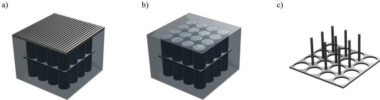
Figure 1: Hybrid thermal management system proposed including immersion single-phase liquid cooling, fin, heat pipes and heat sink: a) overall view including heat sink on top, (b) overall system excluding heat sink, (c) focus on fin and 9 x heat pipes.
