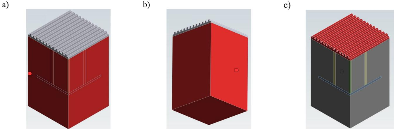
Figure 2: View of the control volume simulated in ANSYS equal to a quarter of the real TMS shown in Figure 1. The external boundary walls are clearly identified: a) symmetry wall, b) insulation wall, c) convection (heat sink) wall.
