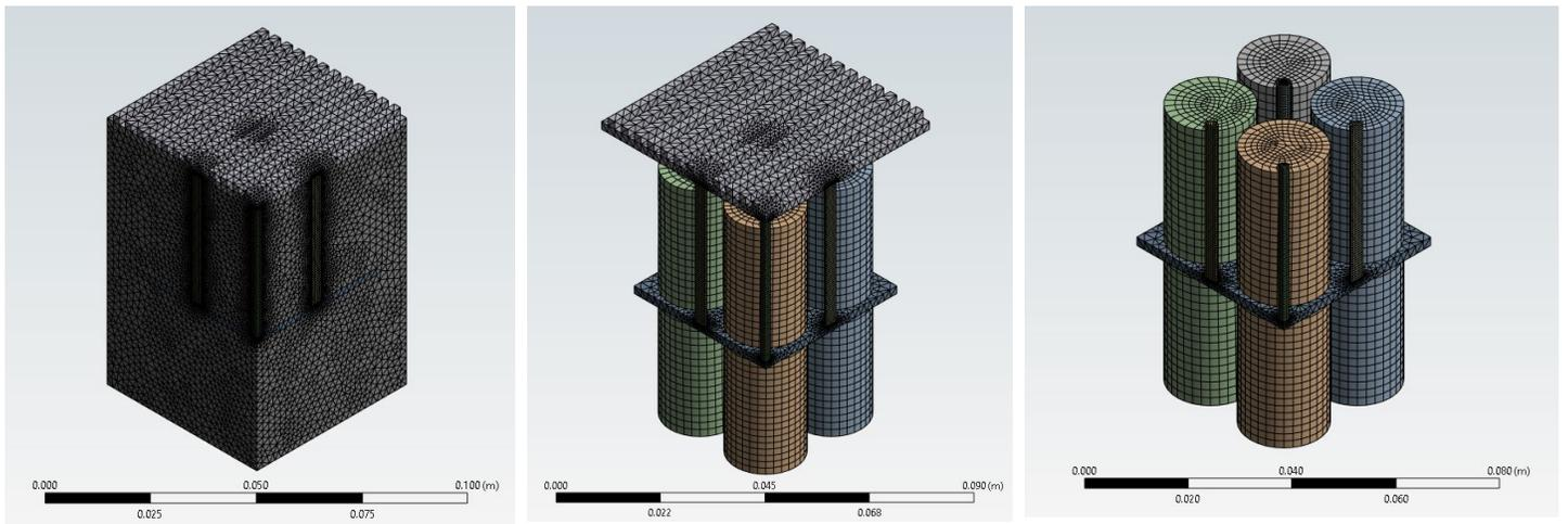
Figure 3: Example of mesh generated in ANSYS, with a specific focus on: a) overall system, b) battery cells, fin, heat pipes, heat sink, c) battery cells, fin, heat pipes.
