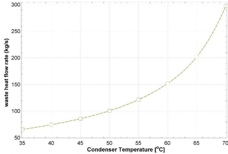
Fig. 5: Impact of the condenser temperature on waste heat mass flow rate
