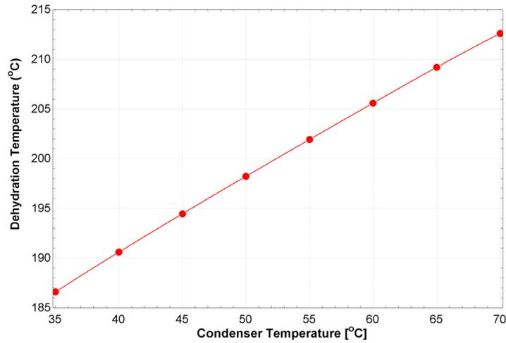
Fig. 3: Dehydration temperature versus condenser temperature
