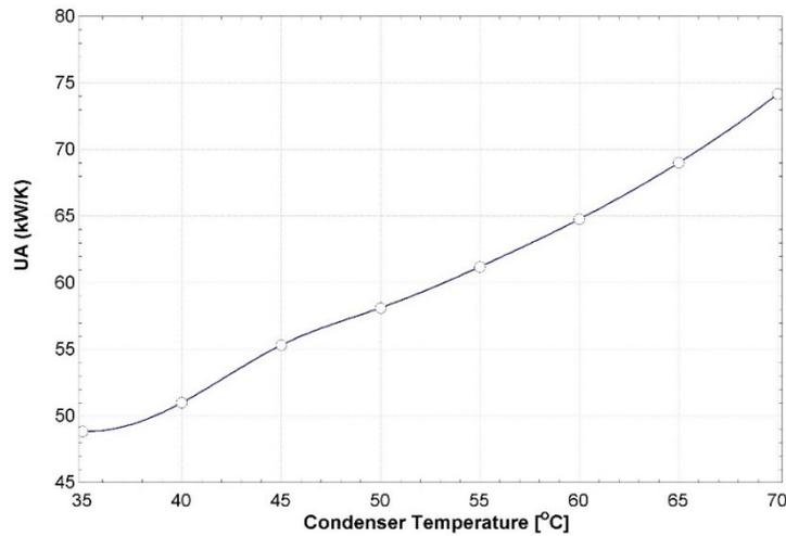
Fig. 6: Impact of the condenser temperature on the size of the waste heat recovery unit
