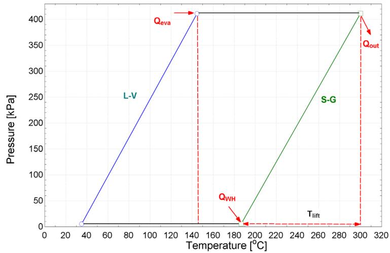
Fig. 2: van't Hoff diagram for the proposed TCHT system.
