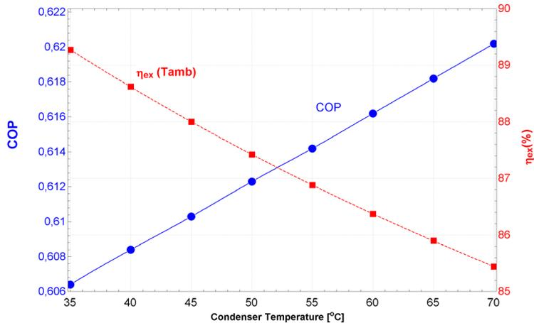
Fig. 4: COPh and exergy efficiency versus condenser temperature
