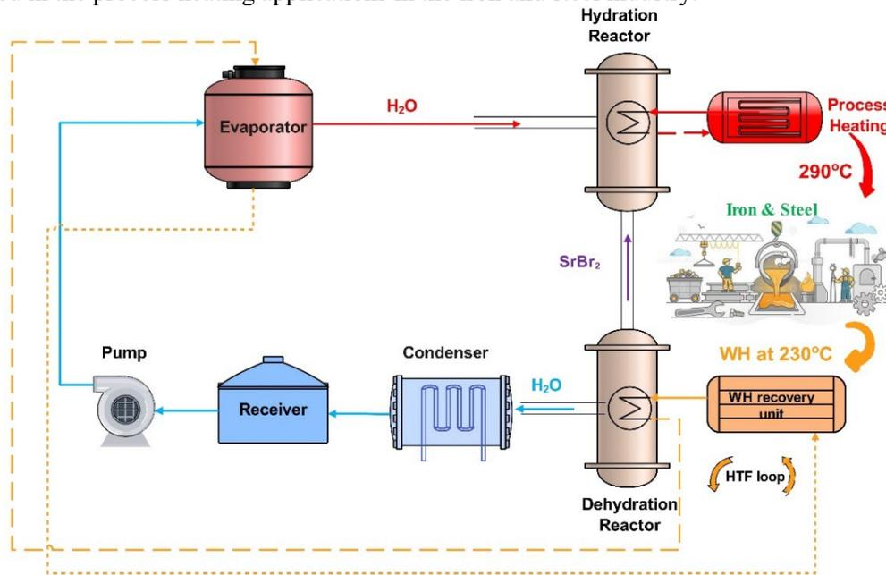
Fig. 1: Proposed TCHT system for heat upgrading in the Iron & Steel industry.
