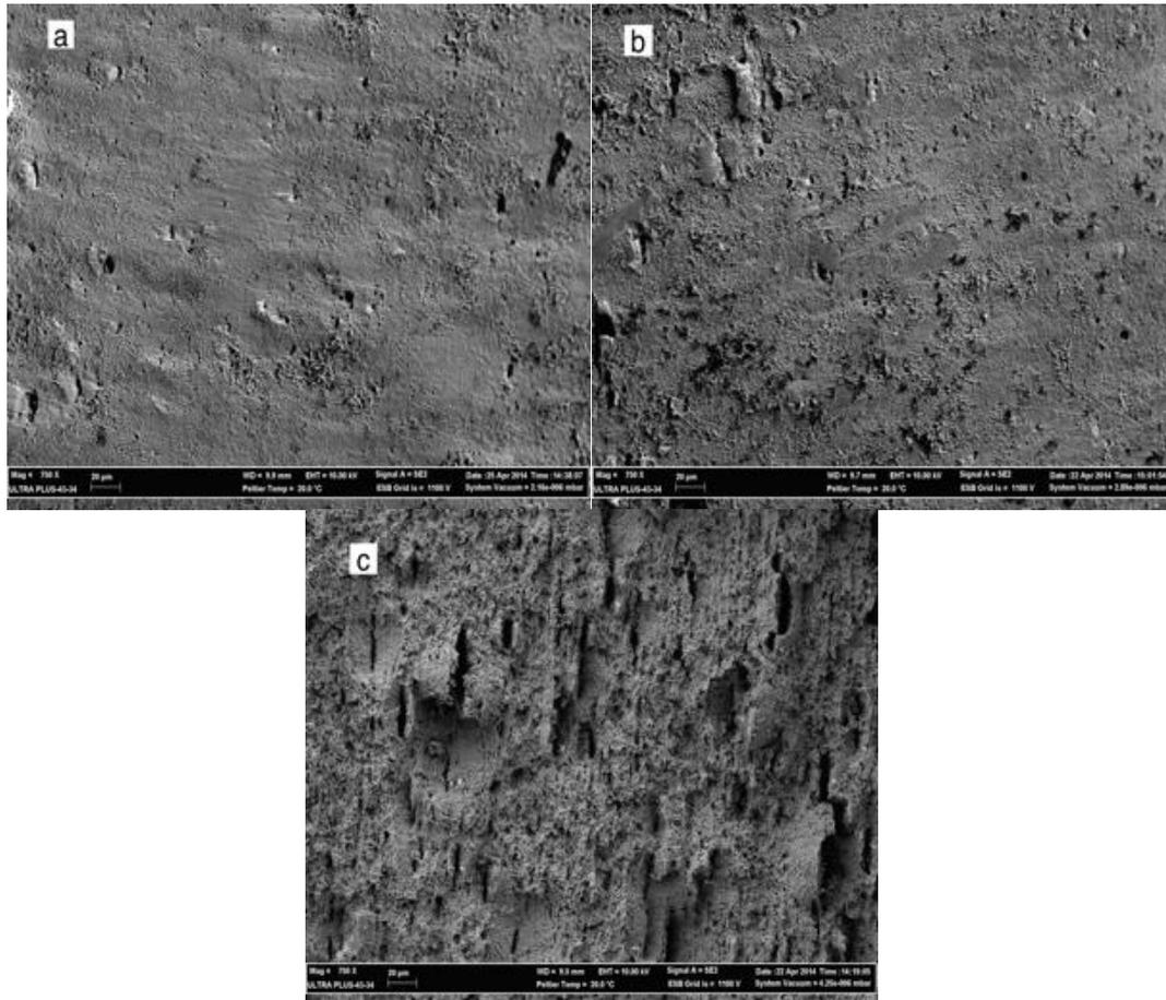
Fig. 5. SEM micrographs of fracture surface of specimens annealed at (a) 900°C, (b) 800°C, (c) 700°C for 150 minute in %50 cold-rolled Fe–24Mn–0.6C high manganese steel.
