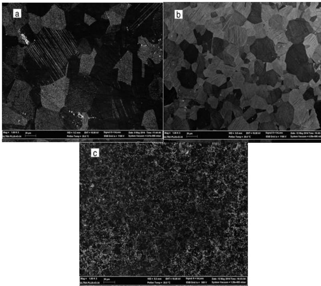
Fig. 1. SEM micrographs of the specimens annealed at (b) 900°C, (c) 800°C, (d) 700°C for 150 minute in %50 cold-rolled Fe–24Mn–0.6C high manganese steel.
