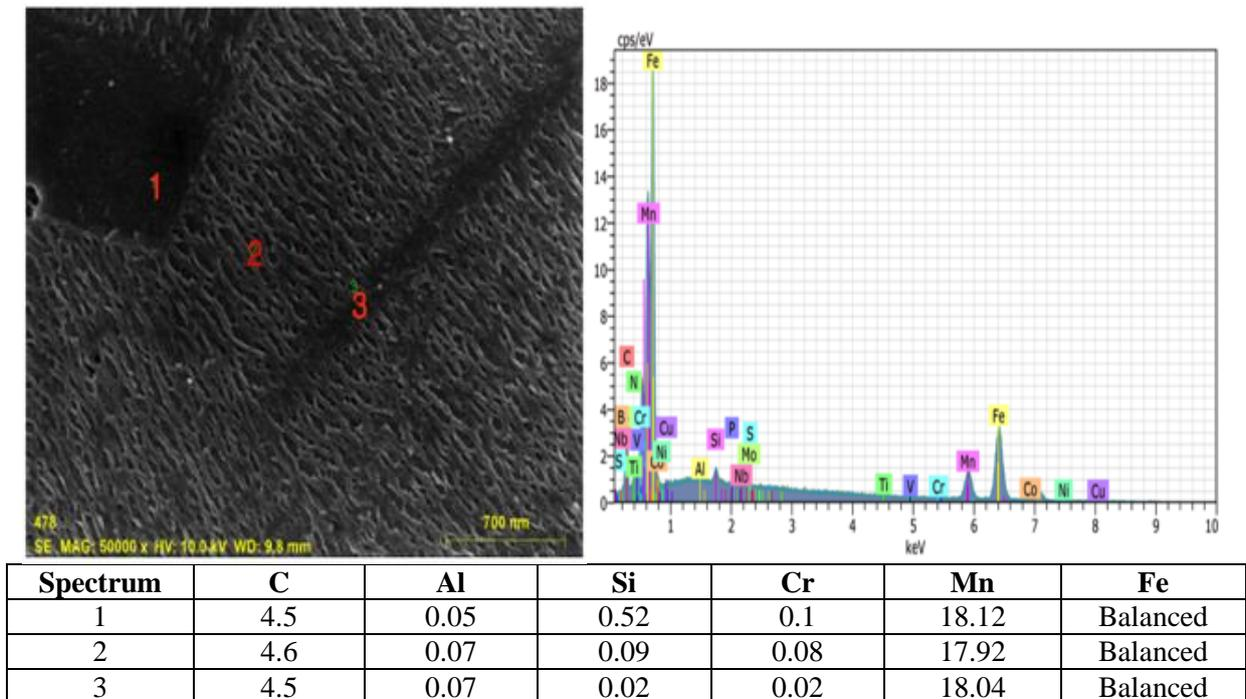
Fig. 3. EDX result of specimen annealed at 800°C.
