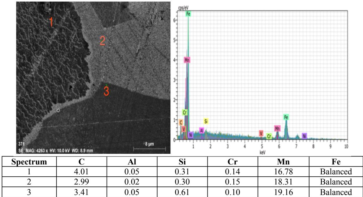
Fig. 2. EDX result of specimen annealed at 900°C.
