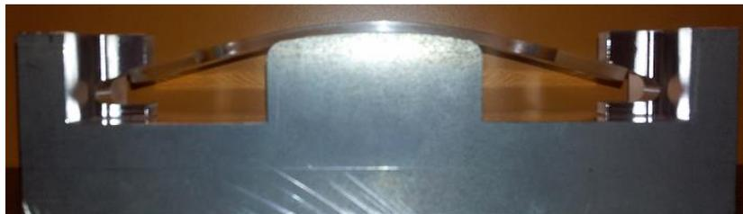
Fig. 1. The preparative for applying the stress to the test object.
