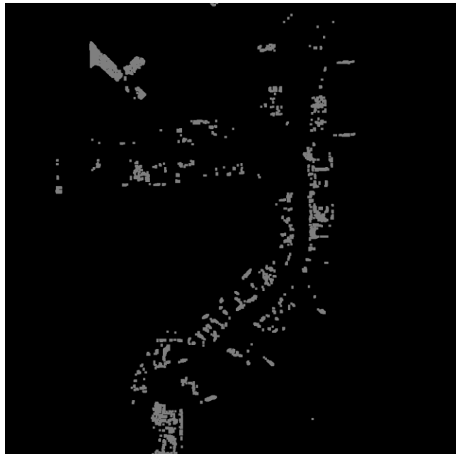
Fig. 2. Result of the identification of the points that correspond to vehicles.
