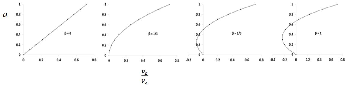
Fig. 1. The down channel velocity profile for various values of  $\beta$ .
