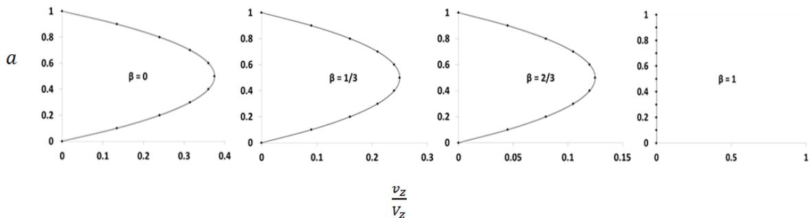
Fig. 2. The axial velocity profile for various values of  $\beta$ .
