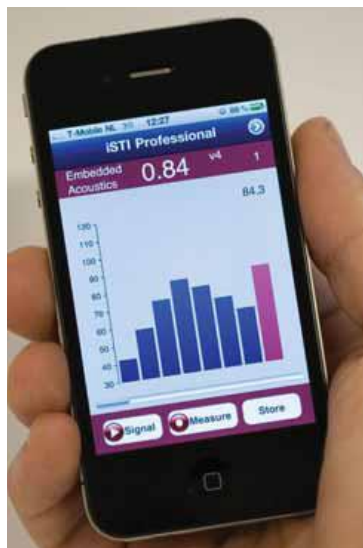
Fig. 4. Example of the STI measurement by the iPhone
