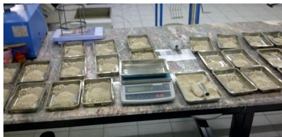
Fig. 2. Aggregate prepared according to Type 2 wearing course
