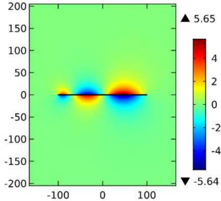
Fig. 4: Effect on pressure of the third natural oscillation mode of the microcantilever on the surrounding fluid (water). The fixed end of the microcantilever is located on the right side of the figure and the scale of this is micrometer. Pressure experimented in the areas close to the microcantilever (Pa). Source: Authors
