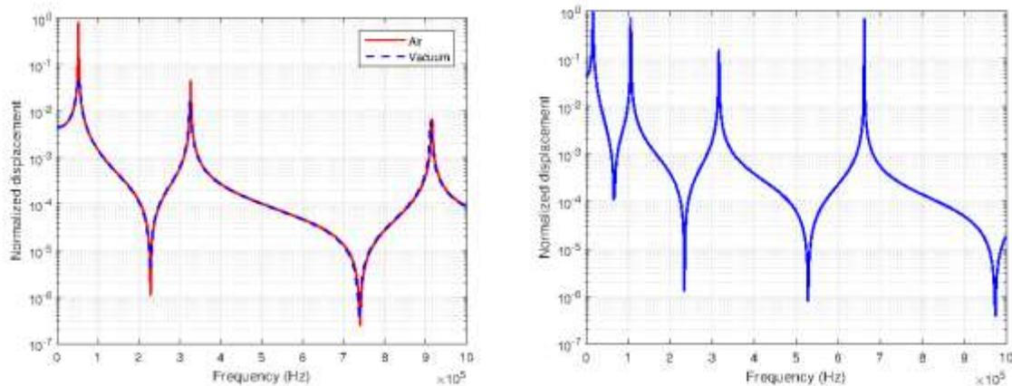
Fig. 3: Frequency sweeps of the microcantilever in different mediums. (a) Frequency sweep in the vacuum and in the air. (b) Frequency sweep in water. Source: Authors.
