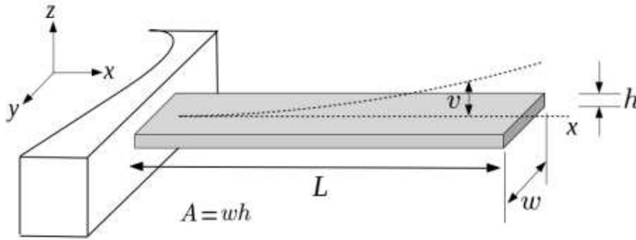
Fig. 1: Scheme of a microcantilever in which the cross section area  $A$ , the length  $L$ , the thickness  $h$ , and the width  $w$ , are shown. Source: Authors.
