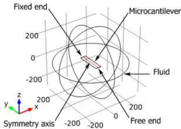
Fig. 2: Geometry used for the simulations of the microcantilever in the presence of a fluid. View of the microcantilever inside the sphere, the symmetry axis, the free end and the fixed end.
