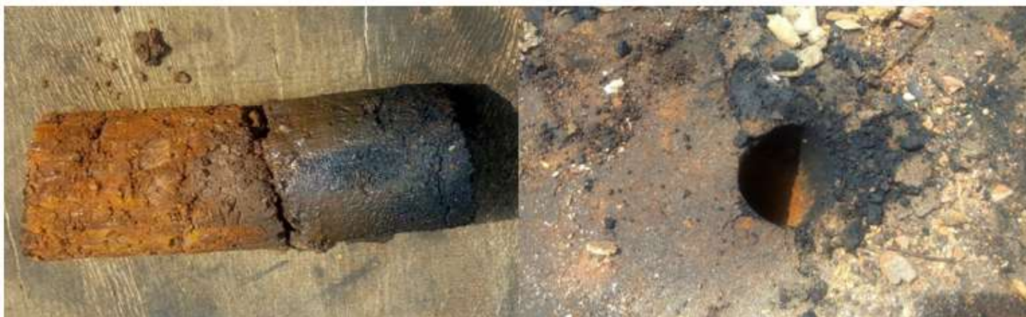
Fig. 1: Core samples of contaminated soil.
