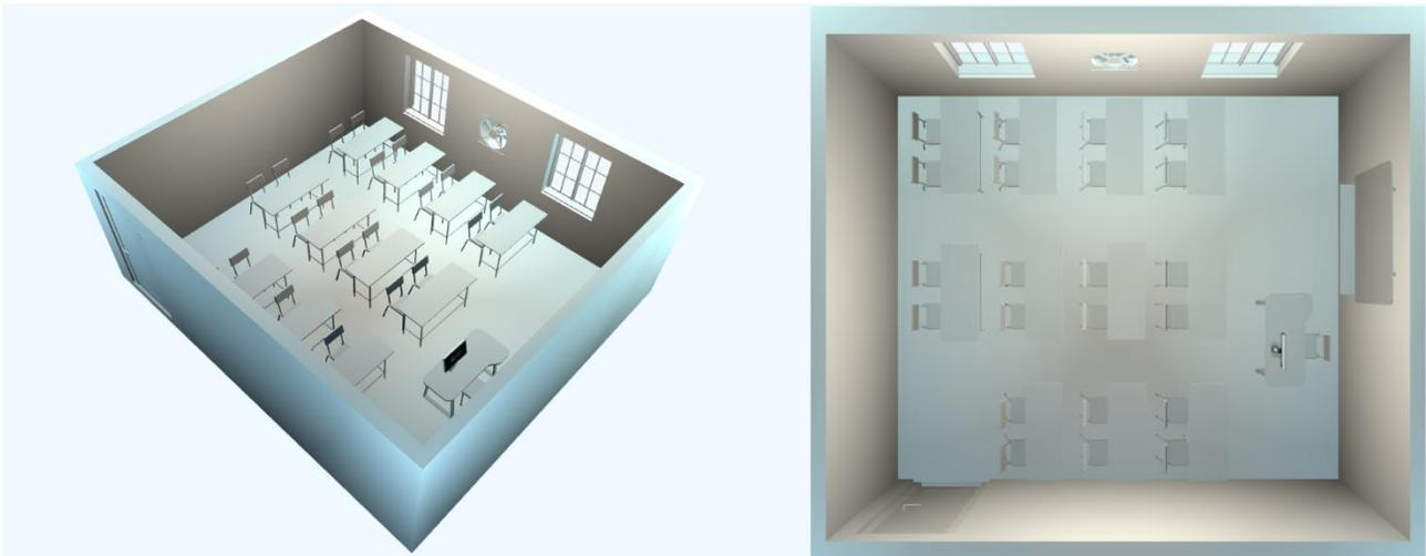
Fig. 1: Solid objects for LBM simulation.
