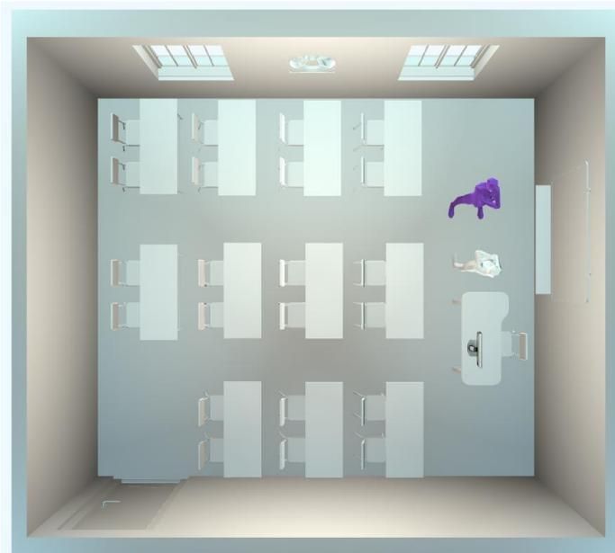
Fig. 3: Case setup for a risk value evaluation. Purple manikin is considered as the infected one.
