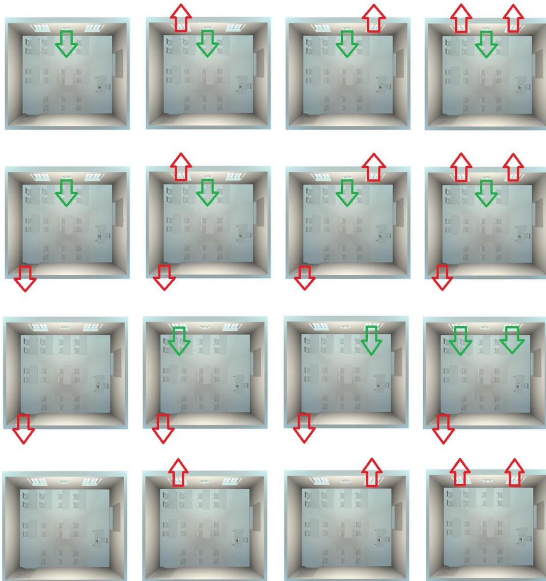
Fig. 2: Boundary conditions and different scenarios, source and sink boundary conditions are green and red arrows, respectively.
