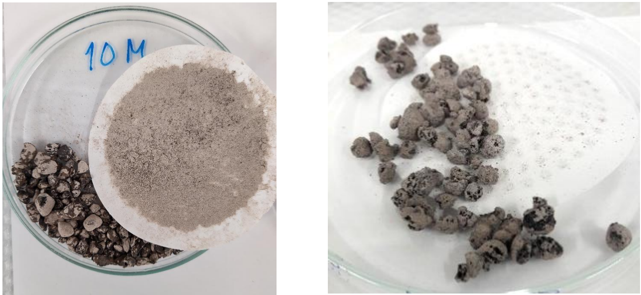
Figure 1: LECA-BFS-based (left, an excluded composition ) and LECA-BFS-based (right, an optimised composition ) adsorbents with BFS functional layer attached after 24h of agitation._
