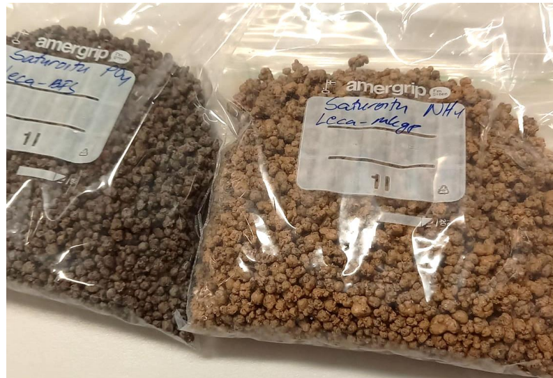
Figure 2: LECA-BFS (left) and LECA-MKGP (right) collected after piloting.
