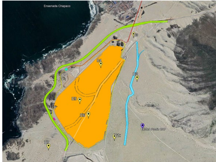
Figure 1. Monitoring points (yellow pins) for particulate material in the sector of the filtered tailings deposit of the Pellet Plant, Huasco (orange area). Lateral road (green), contour channel (light blue).
