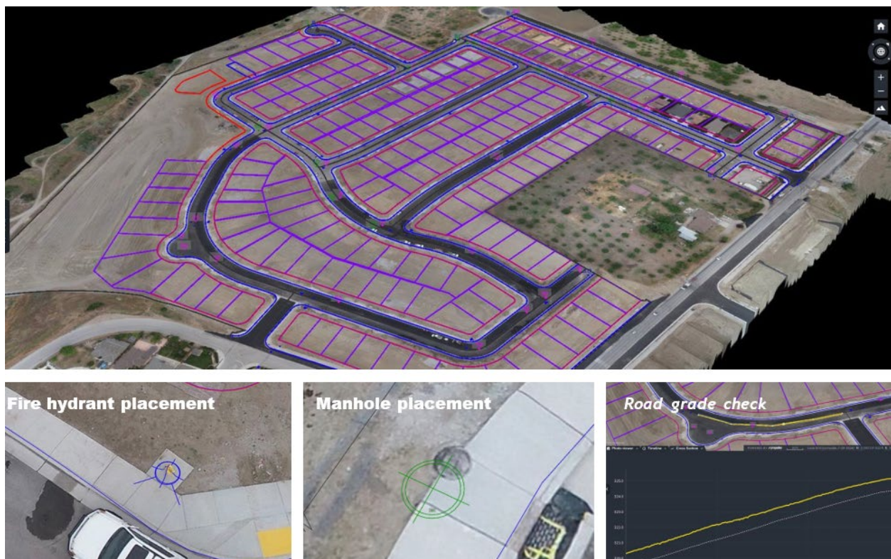
Figure 5. Construction accuracy verification using drone technology [15].
