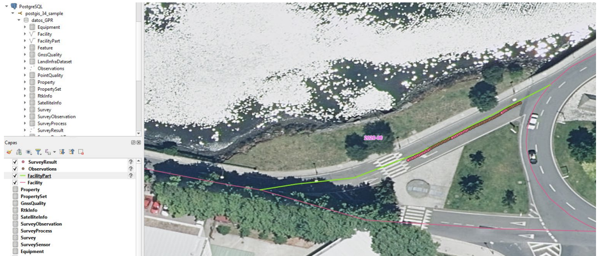
Fig. 8: Example view of model-integrated data on QGIS desktop software.
