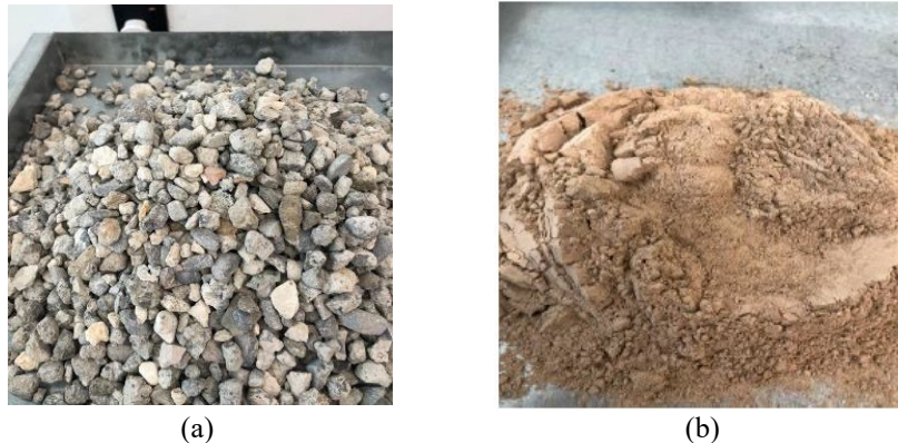
Fig. 1: (a) Recycled Coarse Aggregate (RCA); (b) Ceramic Waste Powder (CWP).
