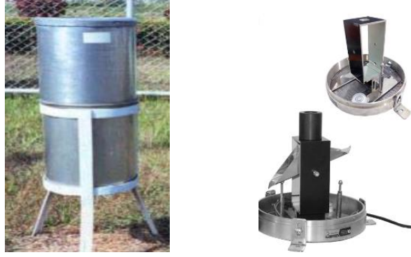
Figure 2: Rain gauge equipment (Source: http://www.cmmet.tmd.go.th/instrument/instruments.php )
