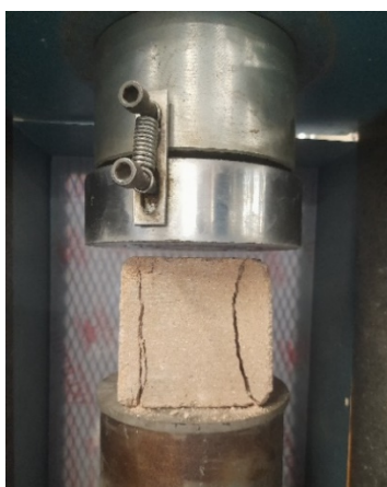
Figure 3: CEB (left) and adobe (right) compressive strength determination
