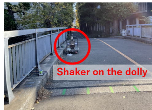
Fig. 13: Configuration of the dolly
