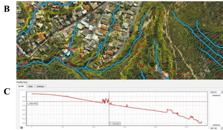
Fig. 3: B - Flow direction of headwater 1 and C - Slope of São Miguel Street. Source: This figure belongs to the authors.
