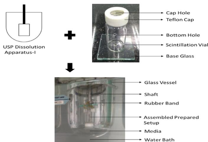
Figure 2: The Modified USP Dissolution Apparatus-I
