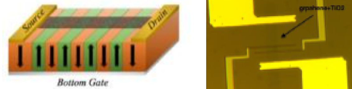
Fig1. Left: Graphene Ferrotronic device architecture where a ferroelectric substrate is periodically poled in order to create a periodic potential; Right: Graphene device for testing width-dependent resistivity.
