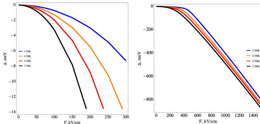
Fig 4. Stark shift dependence on external electric field.
