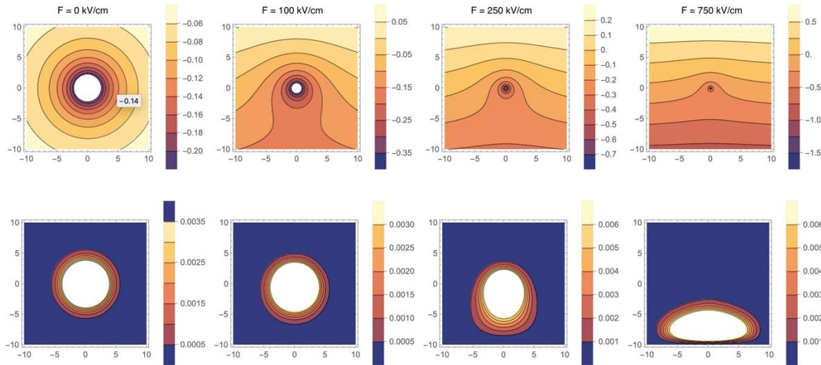
Fig 2. Exciton density distribution (upper row) and potential including electric filed (lower row).  $n=5,5$ .
