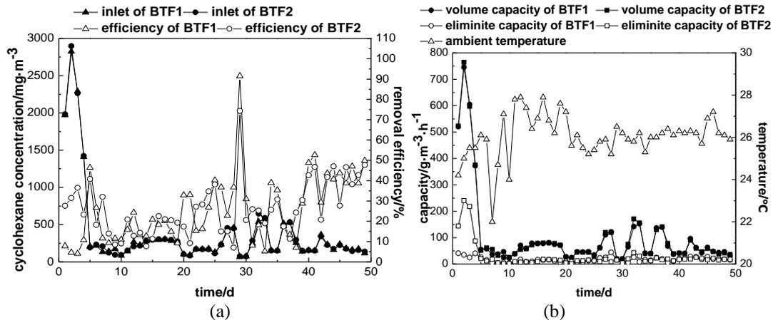
Fig. 3: the change of degradation efficiency for cyclohexane during the start-up period in the activated sludge biofilm BTF ((a) the curve of purification efficiency and the inlet concentration; (b) the curve of removal capacity, volume capacity and ambient temperature)
