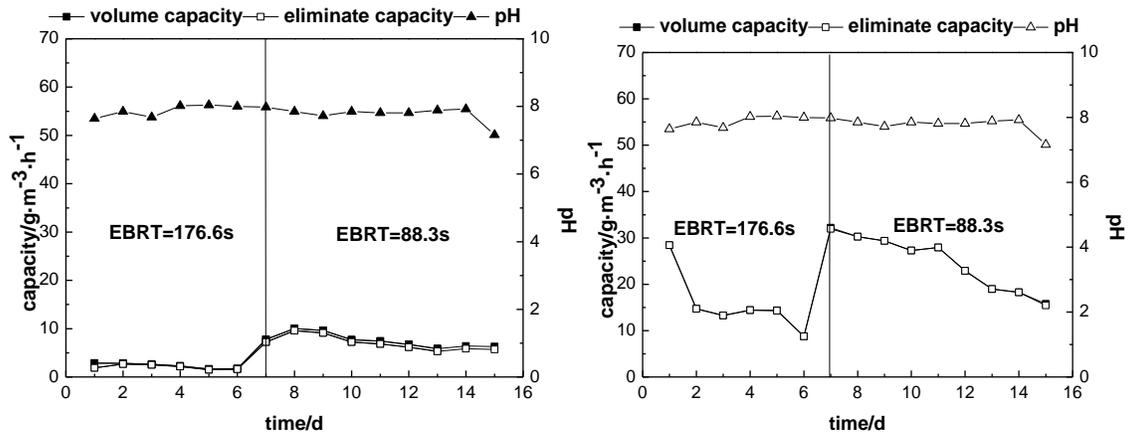
Fig. 7: The curve of cyclohexane and methyl acetate eliminate capacity, volume capacity and solution pH in stable-stage ((a) the curve of cyclohexane eliminate capacity, volume capacity and pH; (b) the curve of methyl acetate eliminate capacity, volume capacity and pH).
