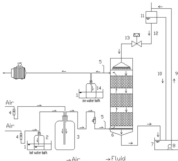
Fig. 1: Schematic diagram of the BTF. 1.thermostatic water bath; 2.toluene solution; 3.air mixed bottle; 4. rotameter; 5. sampling port; 6.BTF; 7. recirculation tank; 8. immersible pump; 9. solution up flow tube; 10.overflow tube; 11.collecting tank; 12.downflow tube; 13.electromagnetism valve; 14.air condensate bottle; 15.air compressor.
