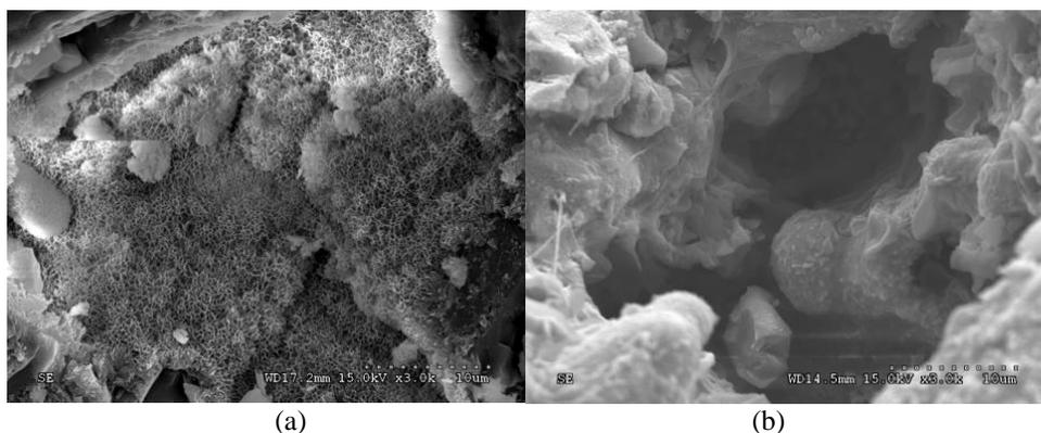
Fig. 2: SEM picture of blank packing ((a) volcanic; (b) ceramic).
