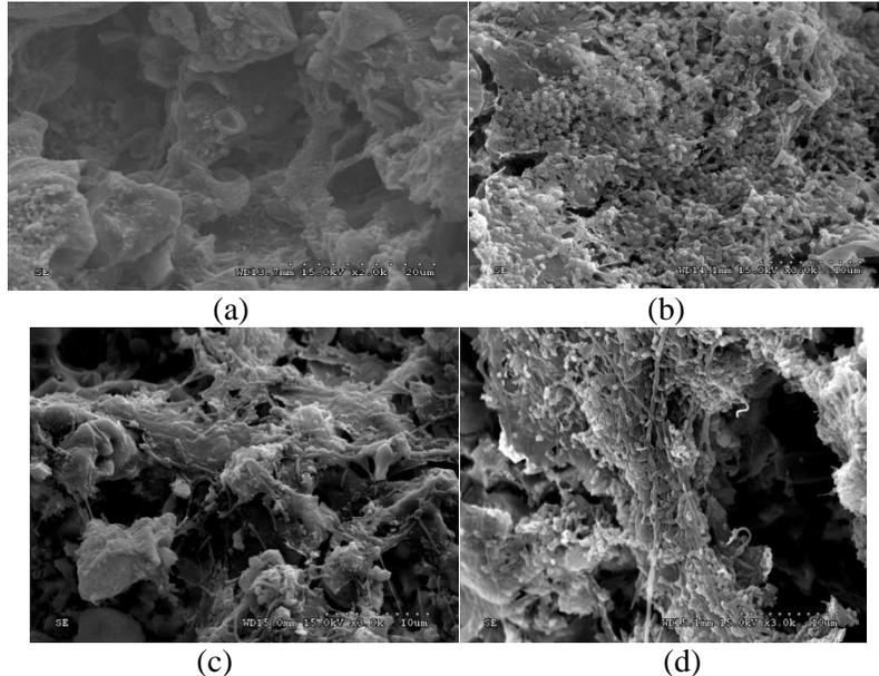
Fig. 5: SEM image of microbial growth on the surface of ceramic before and after film success ((a) blank ceramic, (b) the upper layer, (c) the middle layer and (d) the lower layer).
