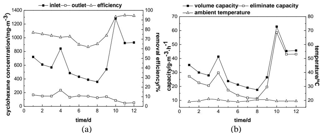
Fig. 4: The curve of REs of cyclohexane during the start-up stage in superiority strain biofilm BTF ((a) the curve of RE and the inlet concentration; (b) the curve of RE, volume capacity and ambient temperature).
