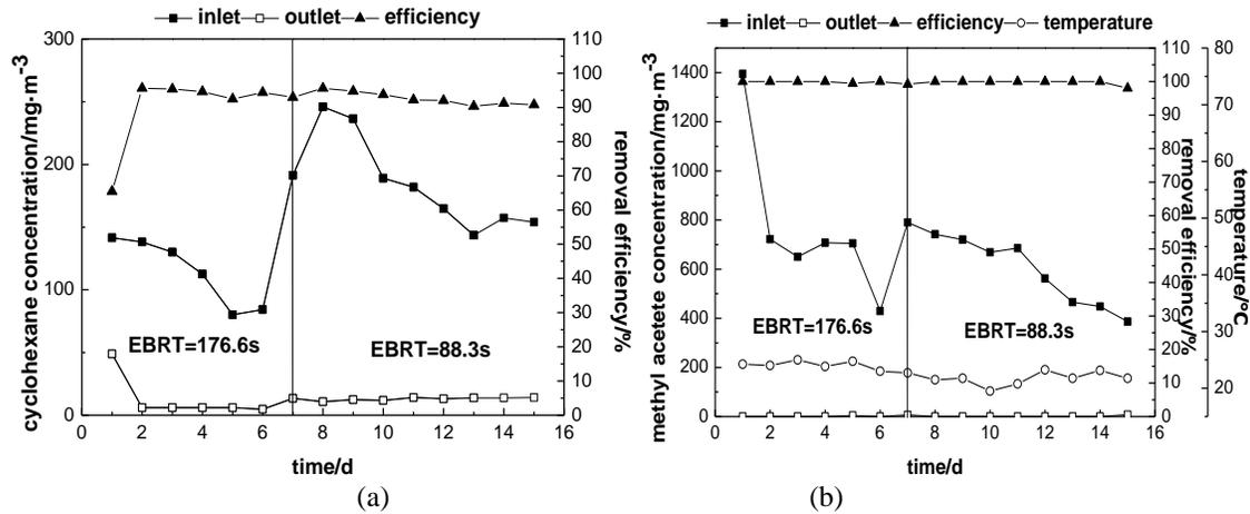
Fig. 6: The change of removal efficiency, inlet concentration and ambient temperature with different EBRT in stable-stage ((a) the curve of cyclohexane RE and the inlet concentration; (b) the curve of methyl acetate RE, inlet concentration and ambient temperature).
