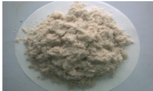
Fig. 6: Chicken feathers after milling.
