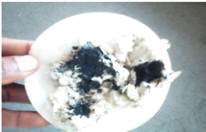
Fig. 8: Bitumen trapped by PCF sorbent during stage 1.
