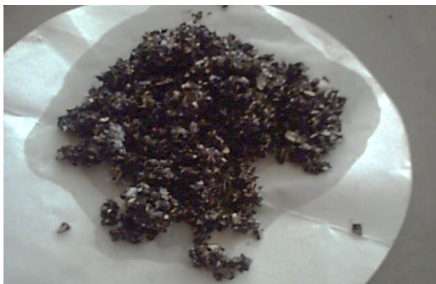
Fig. 9: Bitumen entrapped by PAW seed shells during stage 3.
