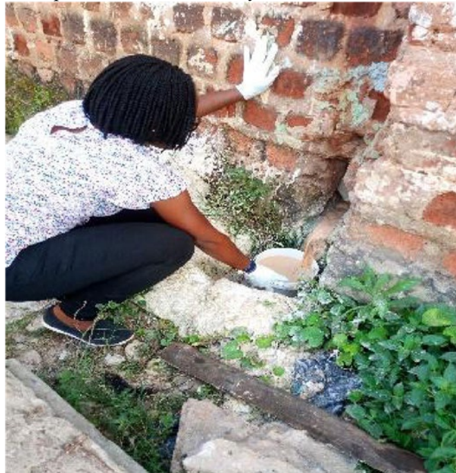
Fig 2: Determining the flow rate using the bucket method
