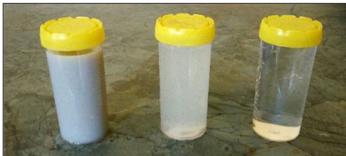
Figure 5: Samples of wastewater from the mixing, sedimentation and filtration units
