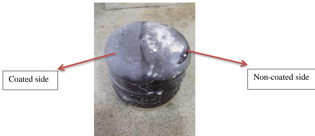
Fig. 3: The insulator that was immersed in the polluted water.
