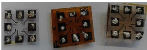
Fig.2. Graphene monolayers on (from left to right) PDMS, Kapton and SU-8 substrates with metallic contacts.
