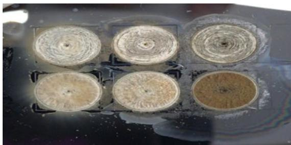
Figure 1. Amount of fiber produced by 20 Watts of power, 1200 KHz of frequency, 0.025 mm pitch, and 10 mm/s of scan speed and 2 loops.
