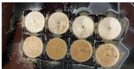
Figure 2. Laser cut Silicon samples prepared. Top row samples were 2 loops laser cut and bottom row were 1 loop laser cut. Both were used for the experiment but the 2 loops (top row) yield better results.
